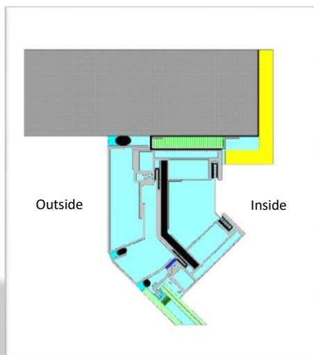
*Here we see a façade junction with a concrete wall. There is a clear run of aluminium from the outside of the mullion to the internal surface.*
