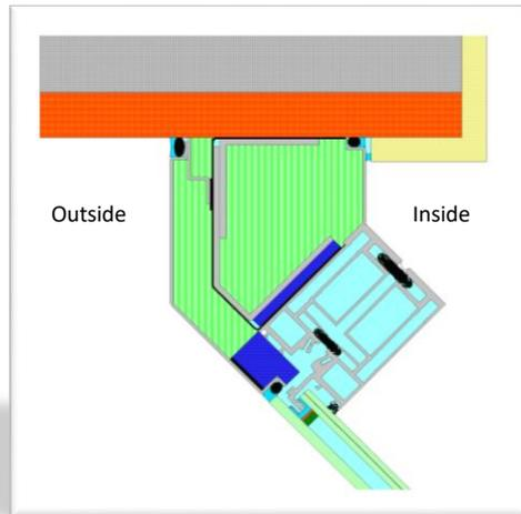
*The façade junction was changed to disrupt the heat flow. The mullion was isolated from the concrete wall and plastic insulation blocks inserted.*
