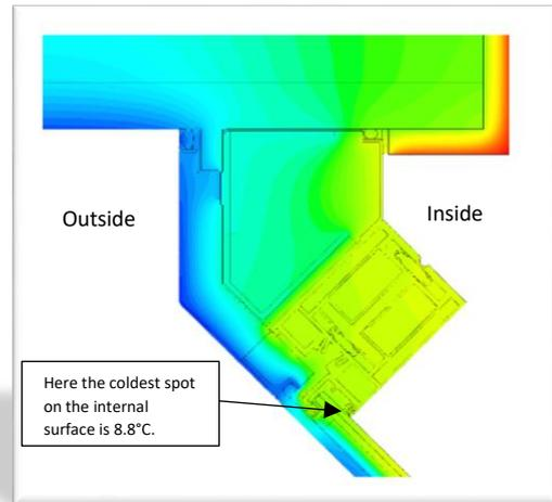
*The internal surface temperature is now much higher and is above the dew point of 6.9°C.*
