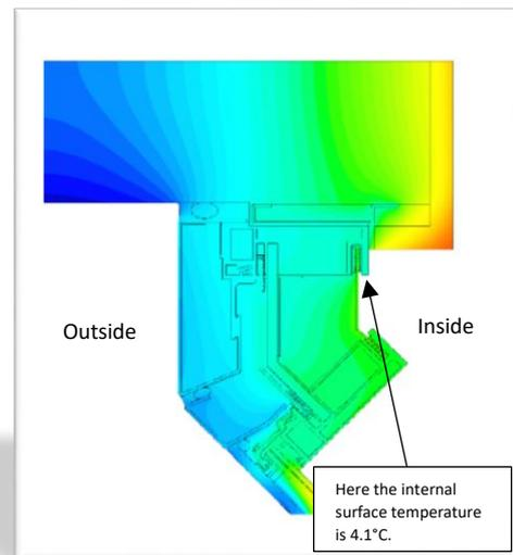
*We can see here that the internal surface temperature of the mullion is very low and so will cause a significant risk of condensation.*
